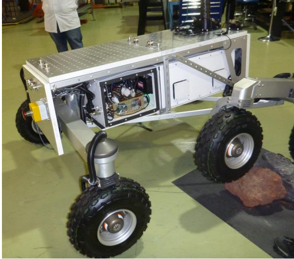
Figure 6: The Mars Exploration Science Rover (MESR) terrestrial prototype with the MPS power system visible in the gold box in the central cavity of the rover
