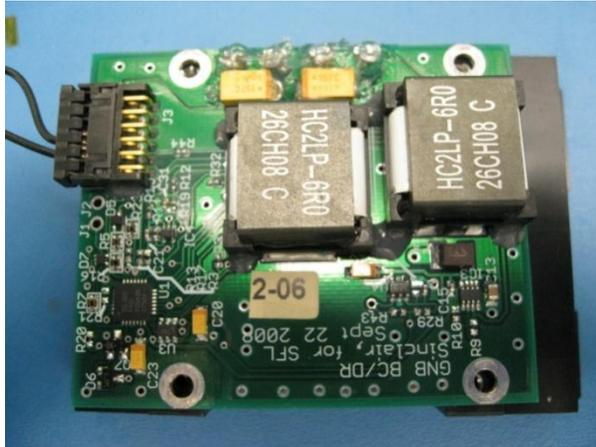
**Figure 9: GNB Battery Charge/Discharge Regulator (BCDR), Top**
