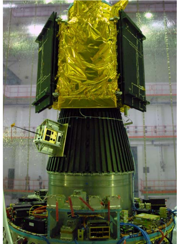
Figure 5. The PSLV-C9 upper stage showing NTS integrated on the XPOD GNB separation system mounted on the Payload Adapter cone.
