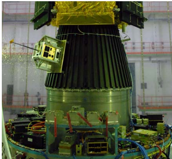
Figure 5. The PSLV-C9 upper stage showing NTS integrated on the XPOD GNB separation system mounted on the Payload Adapter cone.
