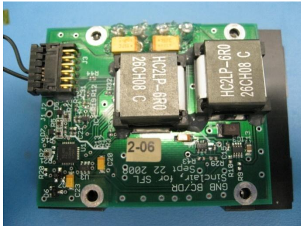
Figure 9: GNB Battery Charge/Discharge Regulator (BCDR), Top
