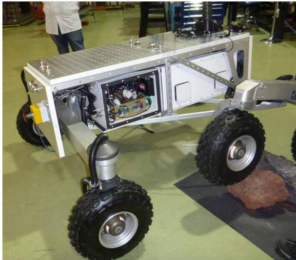
Fig. 6: The Mars Exploration Science Rover (MESR) terrestrial prototype with the MPS power system visible in the gold box in the central cavity of the rover
